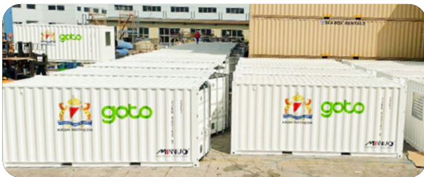
Mobile PSA Plants housed in shipping containers
